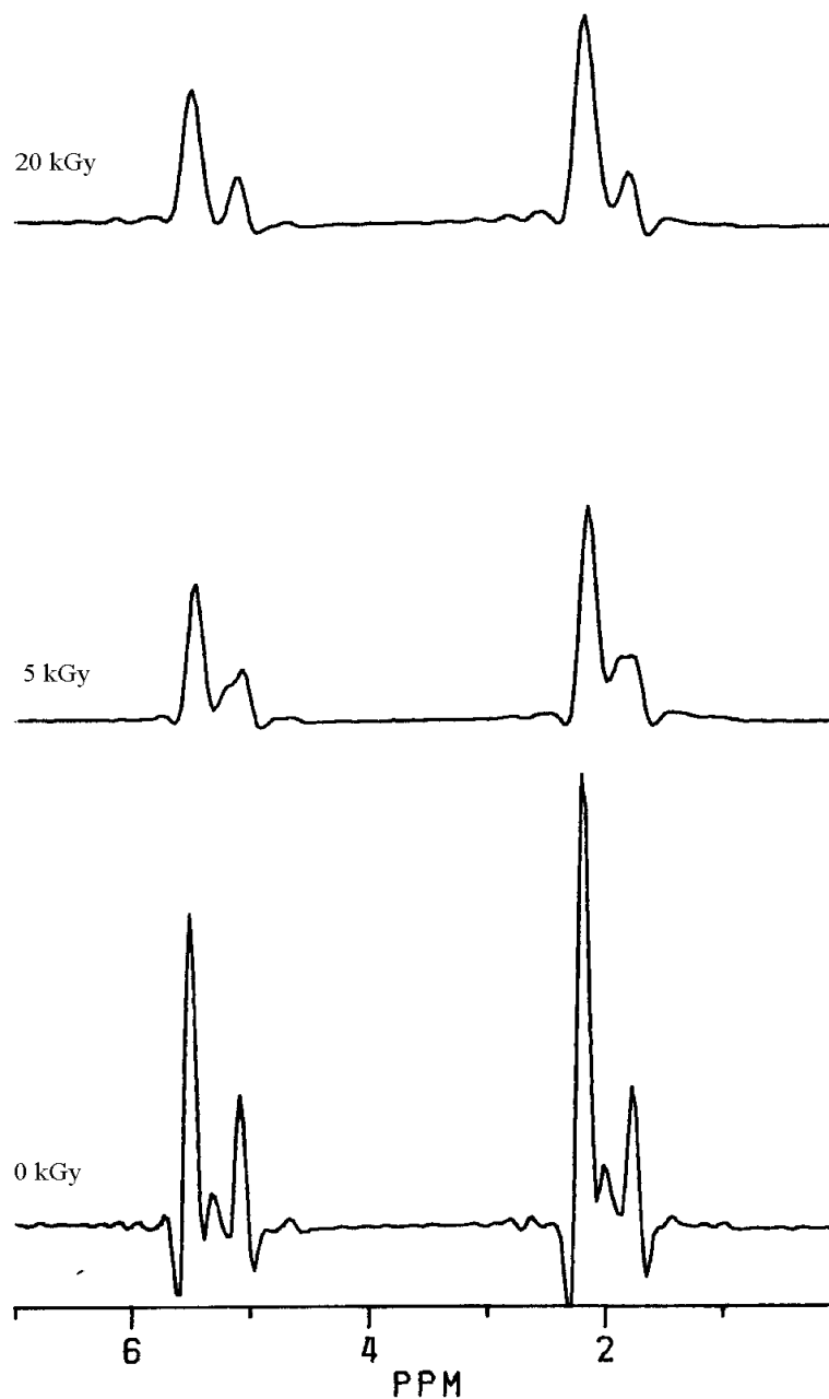
Fig. 8. ^1\text{H} MAS spectra recorded at 200.13 MHz for purified ABS, only the range 7–0 ppm is shown: (bottom) nonirradiated sample; (middle) D = 5 kGy; (Top) D = 20 kGy. A gaussian multiplication function has been applied to improve the resolution enhancement ( \text{LB} = -64 , \text{GB} = 0.4 ).
